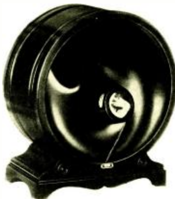
Fig. 4. Application of the unit to the air column. Note that the back of the speaker unit is open so that high frequencies are directly transmitted to the air.
