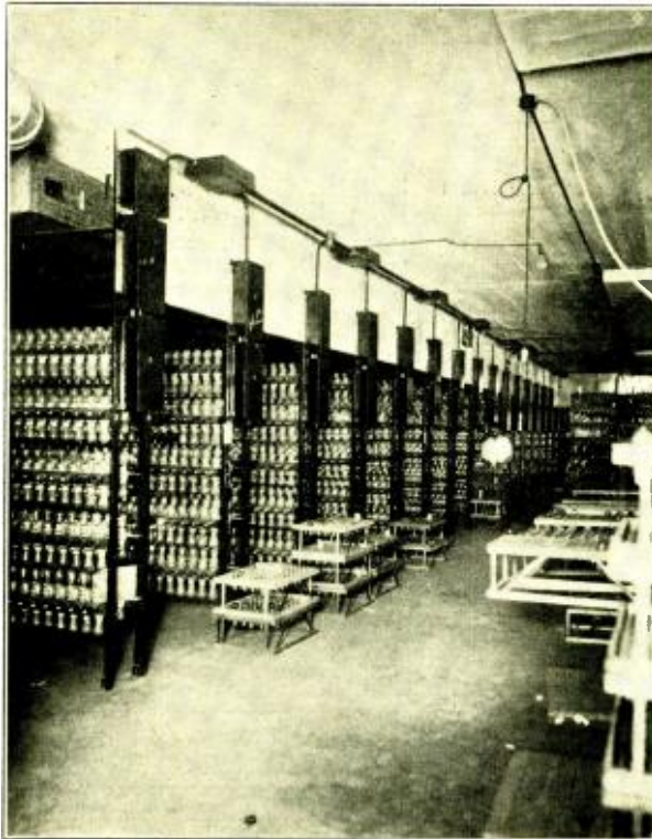
A bank of test racks where the gaseous conduction rectifier tubes are put through their paces. A few of the racks are used principally for conducting life tests.
