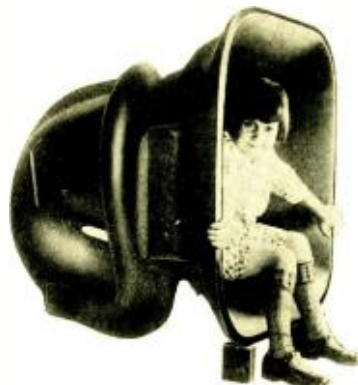
Fig. 3. A giant exponential horn, made in one piece, with an air column ten feet long.
